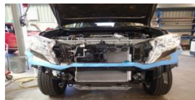
Finished bumper cut looks like this.
