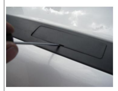
1. Remove cover plates in roof trim (x6) using small flat blade screwdriver.
