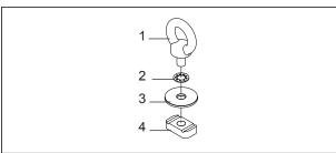
Assemble the shake proof washer and flat washer onto the eyebolt (shake proof washer first). Screw the channel nut onto the eyebolt with the grooves facing the eye bolt.
