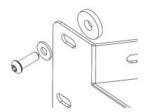
7. Use two M8 buttonhead screws, four M8 washers and two M8 nyloc nuts to fasten the forward jack mount to the Jack mount assembly.
