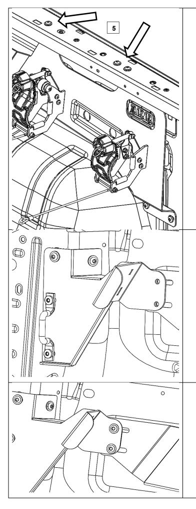
5. Three M8 buttonhead screws, six M8 washers and three M8 Nyloc nuts are used along the top to fit the Jack mount assembly.
