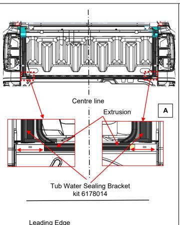
2.4) Measure and position the aluminium extrusion's (668AM002) centre between each of the rear tailgate sealing brackets (A).
