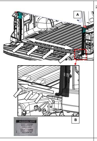
2.2) With the tailgate open, clean the entire length of the rear vertical face of the rear tub floor, between the lower ends of the tailgate sealing brackets as assembled to the vehicle shown at (B) with the alcohol wipe (6602018).
