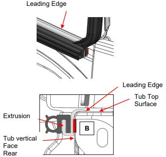
2.5) When positioning the aluminium extrusion, the leading edge of aluminium extrusion should be sitting flat on the top surface of tub and the taped side to the vertical face of the rear edge of the tub's floor (B).
