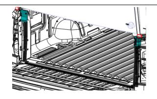
2.6) Check Lower Dust kit is secure and installed correctly. Check tailgate operation by opening and closing it, ensuring the tailgate functions and the seals makes contact to the lower angled face of the tailgate.
